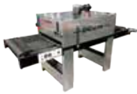
ENCORE #2408-2 230 Volts; 1-Phase 24" Belt Width; 8' Long
