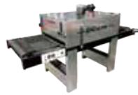
ENCORE #2408-2 230 Volts; 1-Phase 24" Belt Width; 8' Long
